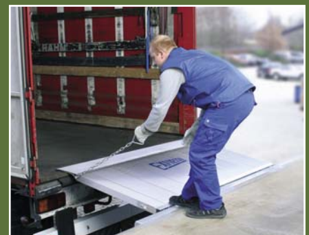
... the leveller is lowered...
